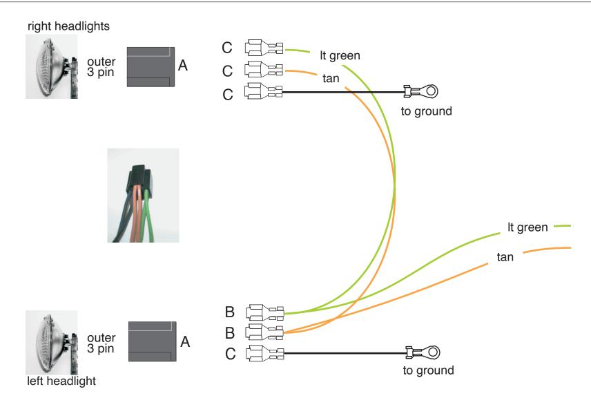
The 1970 Mustang utilized a single headlamp system as opposed to the dual headlamp system used on the 1969 Mustangs. On this sheet, you will find instructions that depict how to connect your headlamps. The function of each of the wires (It. green, tan, and black) remains the same as on the main instruction sheet 510177 page 2, branch 2. AAW recommends that you use both this sheet and the 510177 sheet for installation of your headlamps.
